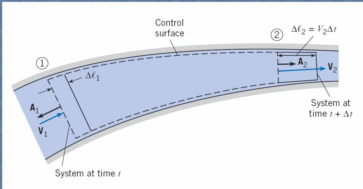
The flow of work done by the system at station (2) is given by
